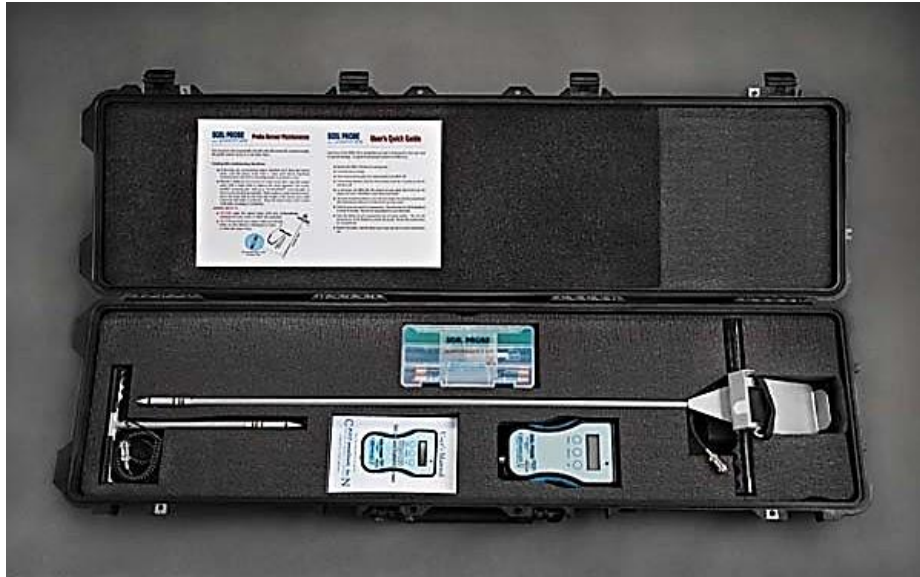
Figure 4.17 Soil pH and resistivity meter (SRM-100, MSES Consultants, Inc.).
