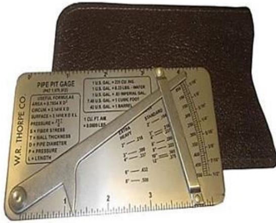
Figure 5.2 Deep pit measurement: (a) pit gage (W.R. Thorpe & Co.); and (b) measurement being performed on Pole TL-1.
