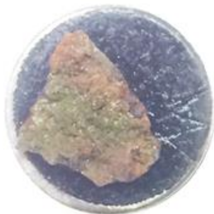
Figure A.15 Loose rust sample from GS fastener region of Pole 11Z-6R at Site 5.
