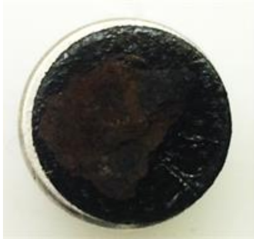
Figure A.5 Pack-rust sample from coating line region of Pole Q3C-2R at Site 2.
