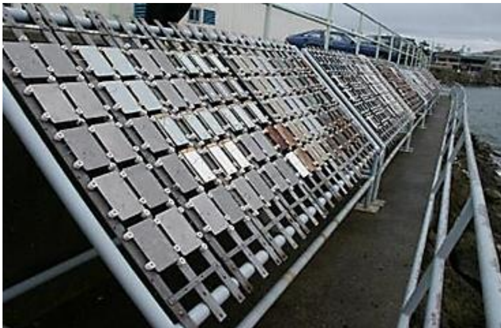
Figure 4.7 Steel panel specimens mounted on inclined rack for corrosion testing in chloride-laden atmosphere (Roberge 2008).
